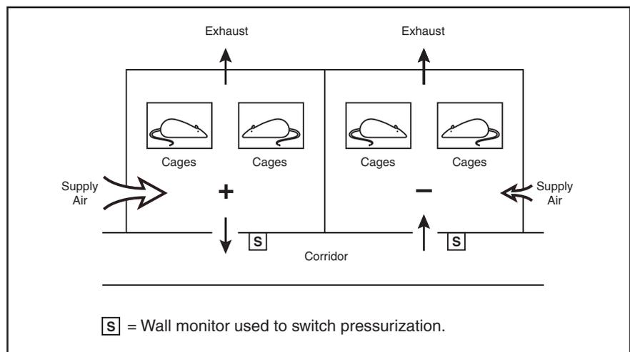
**Planning for flexibility, using switchable holding rooms.** Transgenic facilities generally operate holding rooms under positive pressure. In the event of a contagious outbreak, the rooms may be switched to a containment mode, with the room maintained at a negative pressure.
